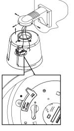
6. Fit and turn the Speed Dome Camera into the slot, locating it in the direction marked on the mounting bracket, and fix it using the rotation control screw.
